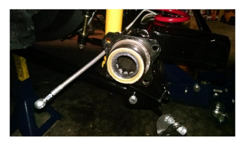
002 - Install new CTS-V Brake Brackets with new Hardware.
