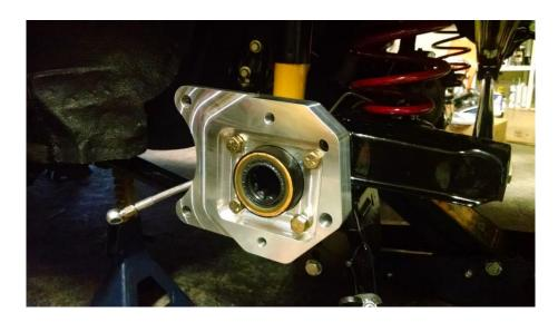
003 - Install new CTS-V Parking Brake Assemblies with new hardware.
