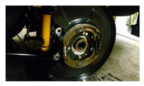
004 – Install new CTS-V Parking Brake Cable Brackets, Parking Brake Conversion Cables, and Stainless Steel Brake Hoses. Latch the Parking Brake Cables onto the Parking Brake Levers. Reinstall the Axles, C-Clips\*, and the Differential Cover.
