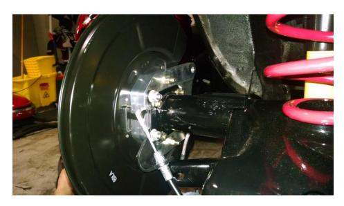
005 – Install Rotors, Calipers, and Brake Pads. Connect the new Stainless Steel Brake Hose to the Caliper with new Copper Bushings and Caliper Bolt. Bleed Rear Calipers and Reinstall Wheel.
