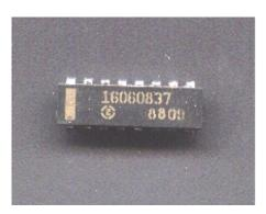
The CALPAC marking used for identification is the 8-digit part number printed on the CALPAC body.
