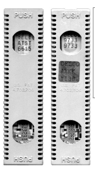
Note: The markings on the left MEMCAL are printed on a label that is affixed to the PROM inside the MEMCAL assembly.
