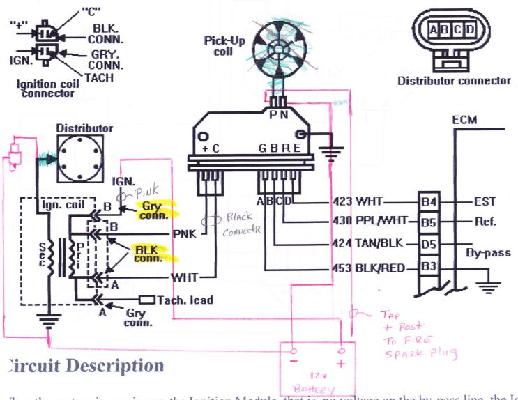
Then the system is running on the Ignition Module, that is, no voltage on the by-pass line, the Ignition Then the rpm for EST is reached (about 400 rpm), and by-pass voltage applied, the EST should no lot the by-pass line is open or grounded, the ignition module will not switch to EST mode, so the EST the EST line is grounded, the ignition module will switch to EST, but because the line is grounded to
