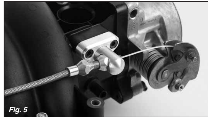
GM LS1 Shown with Lokar Throttle Cable Bracket
