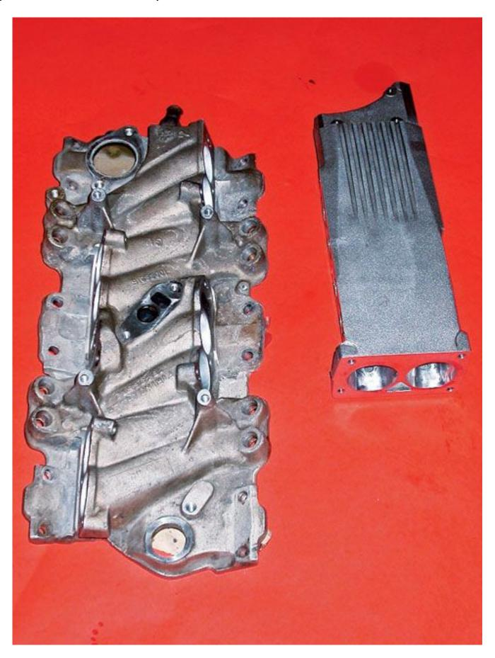
Extrude Hone also worked its magic on the factory L98 lower intake and upper plenum.
