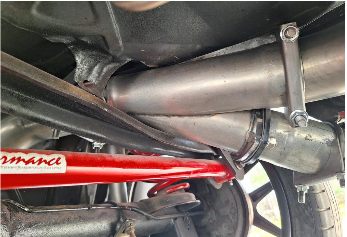
This is a pic of the cutout (you can see the 90 degree pipe going over the axel at the left of the pic) with a piece of u-bend pipe heading to the muffler (top right of pic) and the exhaust reducer which goes to the passenger side exhaust pipe (center right of pic).
