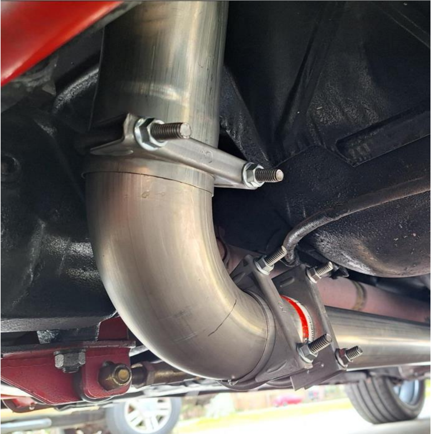
Here is a better picture of the piece I cut from the u-bend pipe mated up to the 3" ID to 3" ID coupler on the right and the 90 degree pipe above it.
