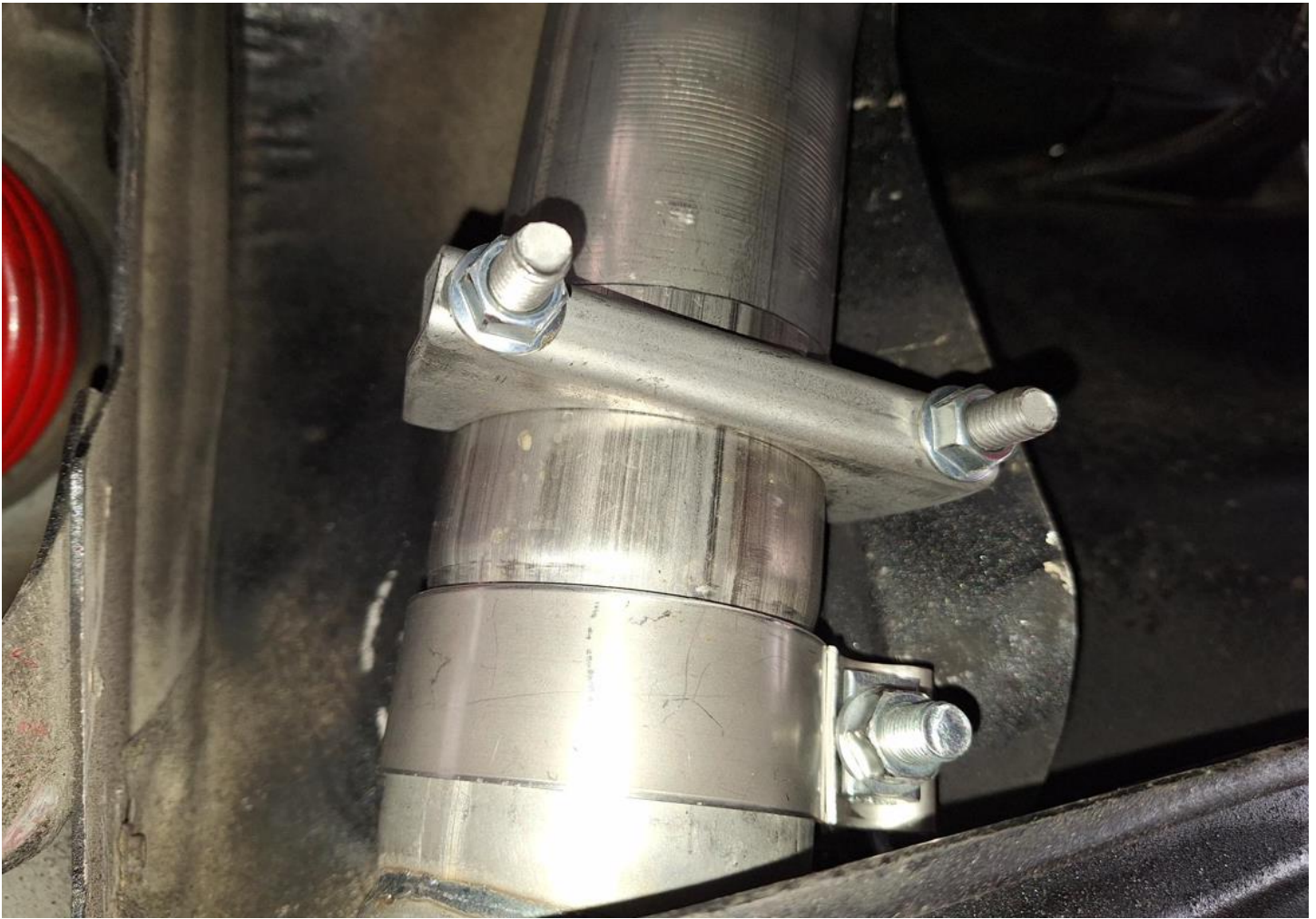
This is a pic of the 90 degree pipe coming from over the axle at the top to the cutout. I had to cut a piece from the 'sleeve' end of a u-bend pipe to give the 90 degree pipe enough clearance over the axel.
