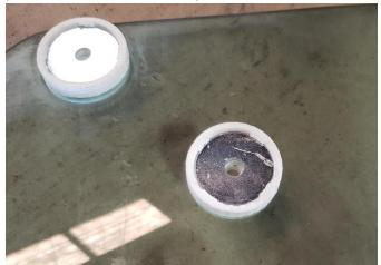
The "Retaining" piece is then pressed into the other side; should snap into place and hold both sides together.
