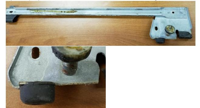
8. With everything clean and disassembled, install any needed replacement plastics into the door. "Bushing" piece with metal washer goes on the outside-facing side of the glass, and should be pushed in first (will sit loosely)
