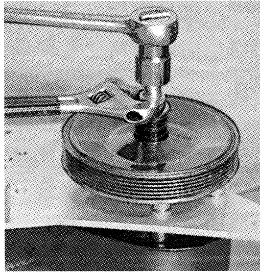
Photo 4-8 / P/S pump pulley reinstallation
