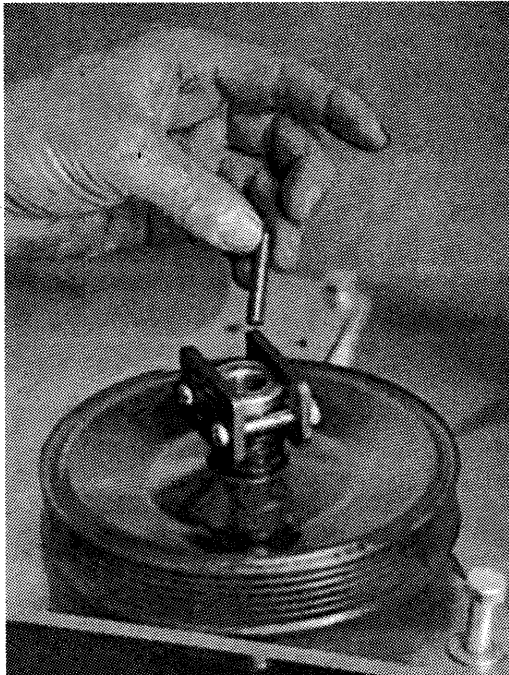
Photo 3-6 / Ball bearing and pin insertion
