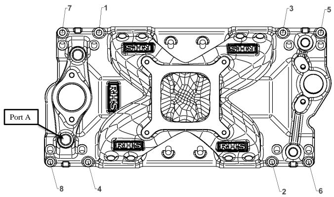
6. Install carburetor/throttle body, distributor and appropriate coolant lines and sensors. Properly plug any unused ports.
