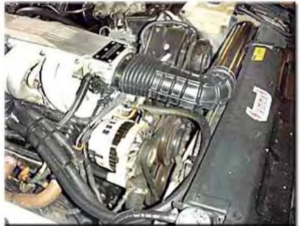
This is what the stock V-belt setup looks like - cluttered, difficult to work on (too many awkward brackets) and the belts tend to squeal.
