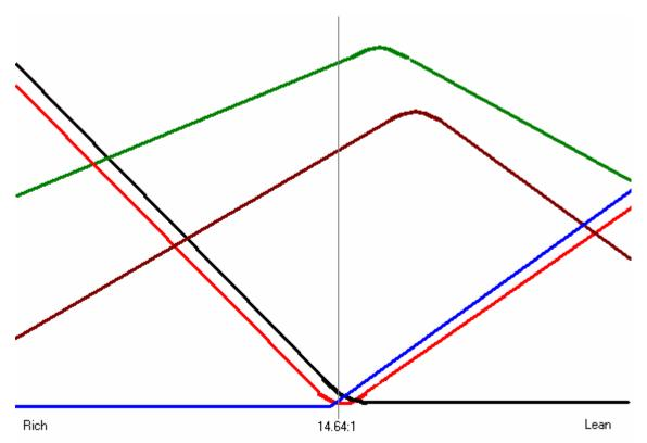
As the air/fuel mixture approaches 14.64:1, the high combustion temperatures (2500 degrees and higher) inside the combustion chamber cause the nitrogen and carbon to compete for oxygen. This prevents perfect combustion from taking place inside the combustion chamber.
