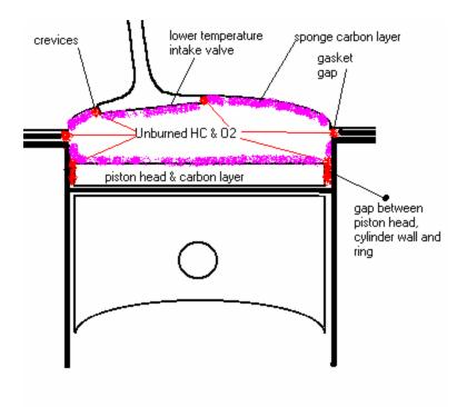
During the compression stroke, air and fuel "hide" in the sponge carbon that forms inside the combustion chamber. The flame front of combustion is quenched or snuffed out as it approaches this carbon layer and the comparatively cool surfaces of the combustion chamber. Any gap, crevice or carbon layer serves as a hiding place for air and fuel.
