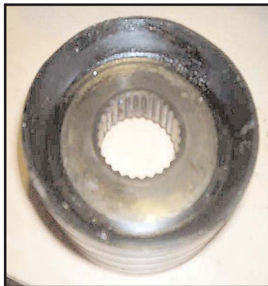
During reassembly, shims are placed under the side gear and the top of the cone. [Side gears are the two large gears and the spider gears are the (four
