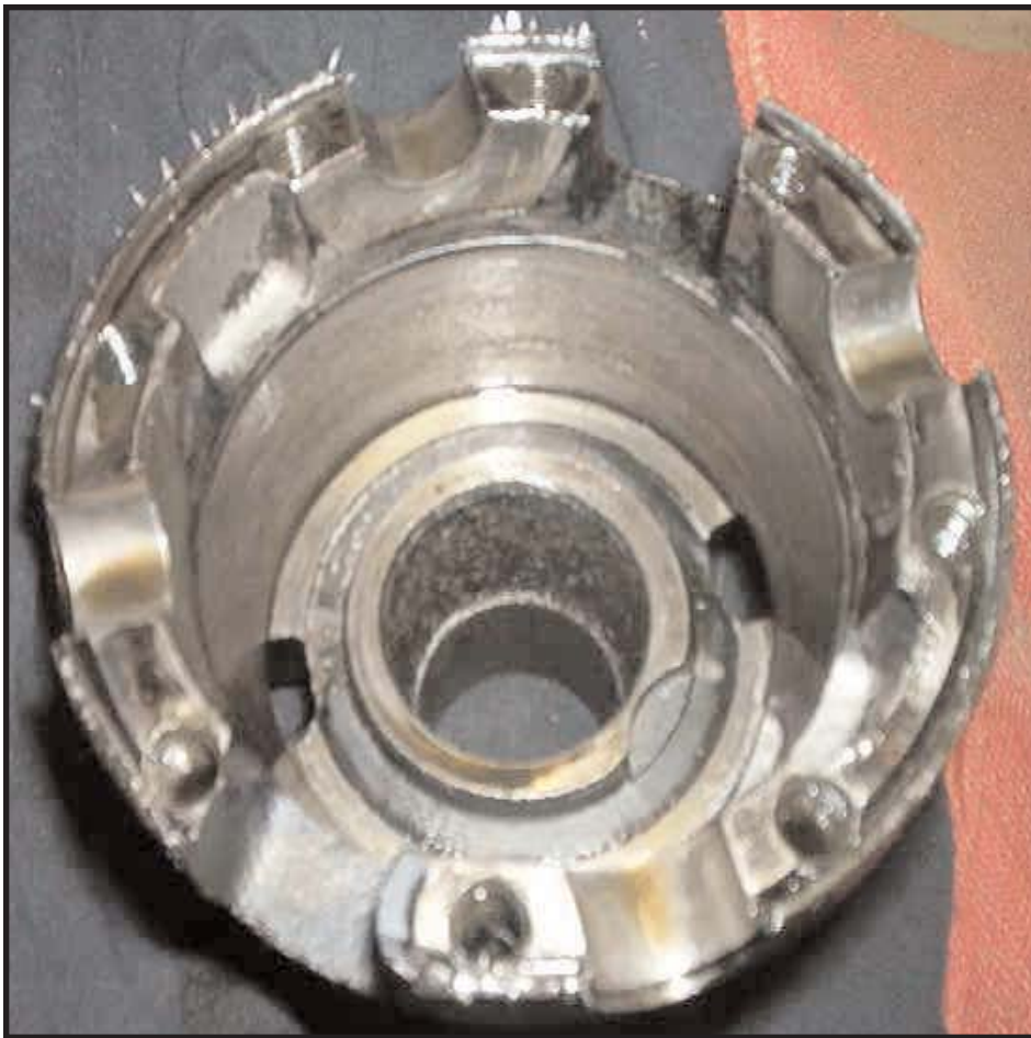
Inside the case housing -- shows why worn cones would quickly bottom out.
