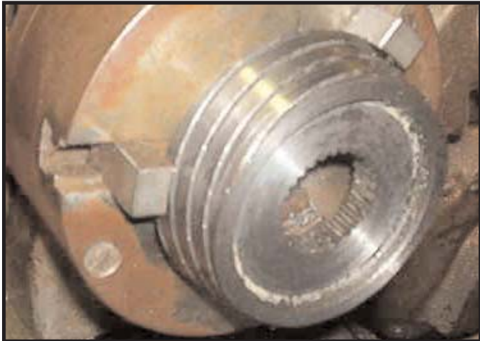
Chucked -- during this repair, not much was taken off the cone on the lath.
