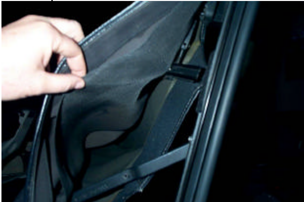
Figure 1: Shown with no flip rod. Notice the #2 bow is still nearly resting on the side seal (top lining pulled back to show the #2 bow).
