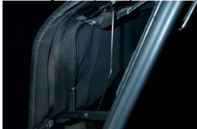
Figure 2: Shown with flip rod installed. Notice the #2 bow is now raised by the flip rod as the top is lowered.
